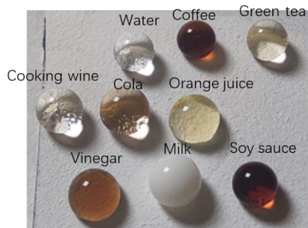
Figure 6. Morphology diagram and CA of different liquids on superhydrophobic surface, morphology diagram.
