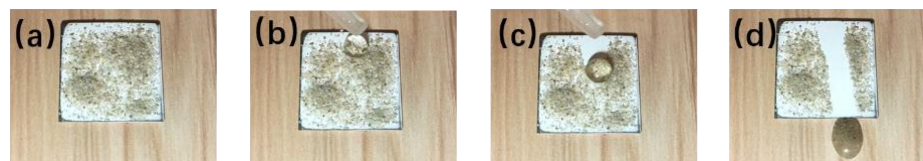
Figure 11. Self-cleaning process of superhydrophobic coating surface: (a) sand was spread on the surface of the coating, (b) sand adhering to the surface of the coating migrates to the surface of the droplets, (c) the water droplets roll off and carry away the sand from the surface, and (d) the surface restores to its original clean state.
