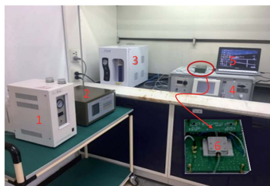
Fig. 4 Sensor measurement system (1-hydrogen generator, 2-flame photometric detector, 3-air generator, 4-CEES generator, 5-PC, 6-prepared SAW sensor system).
