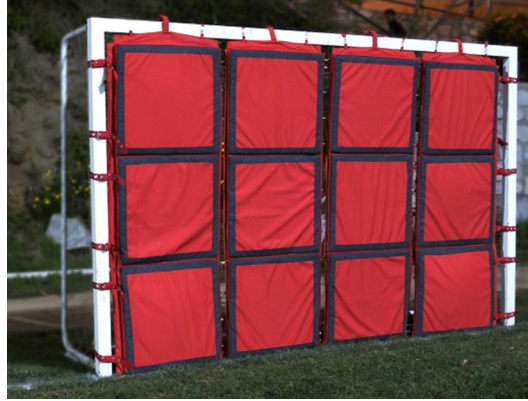
Fig. 4 Picture of the electronic goal developed in this work mounted on an iron goal
