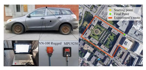
Figure 7. Dynamic experiment's equipment and the experiment's path.
