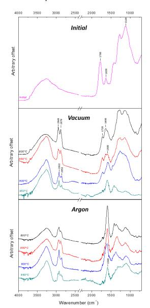
Figure 2. FTIR spectra of initial and annealed DND from 800 °C to 950 °C for both atmospheres.
