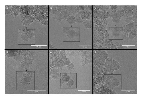
**Figure 5.** HR-TEM images of DND: (**a**–**c**) initial particles; (**d**) 800 °C 4 h; (**e**,**f**) 950 °C 4 h. Images recorded near to Scherzer defocus are provided into insets.
