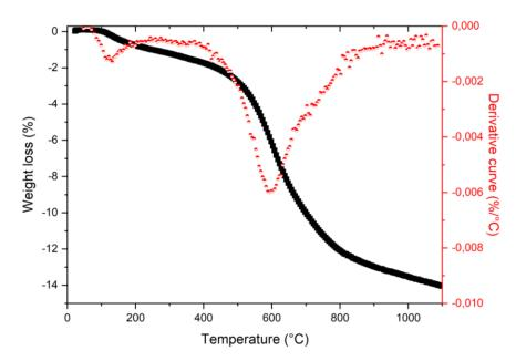
**Figure 1.** TGA spectra of initial DND annealed under argon atmosphere (black) and TGA derivative curve (red).
