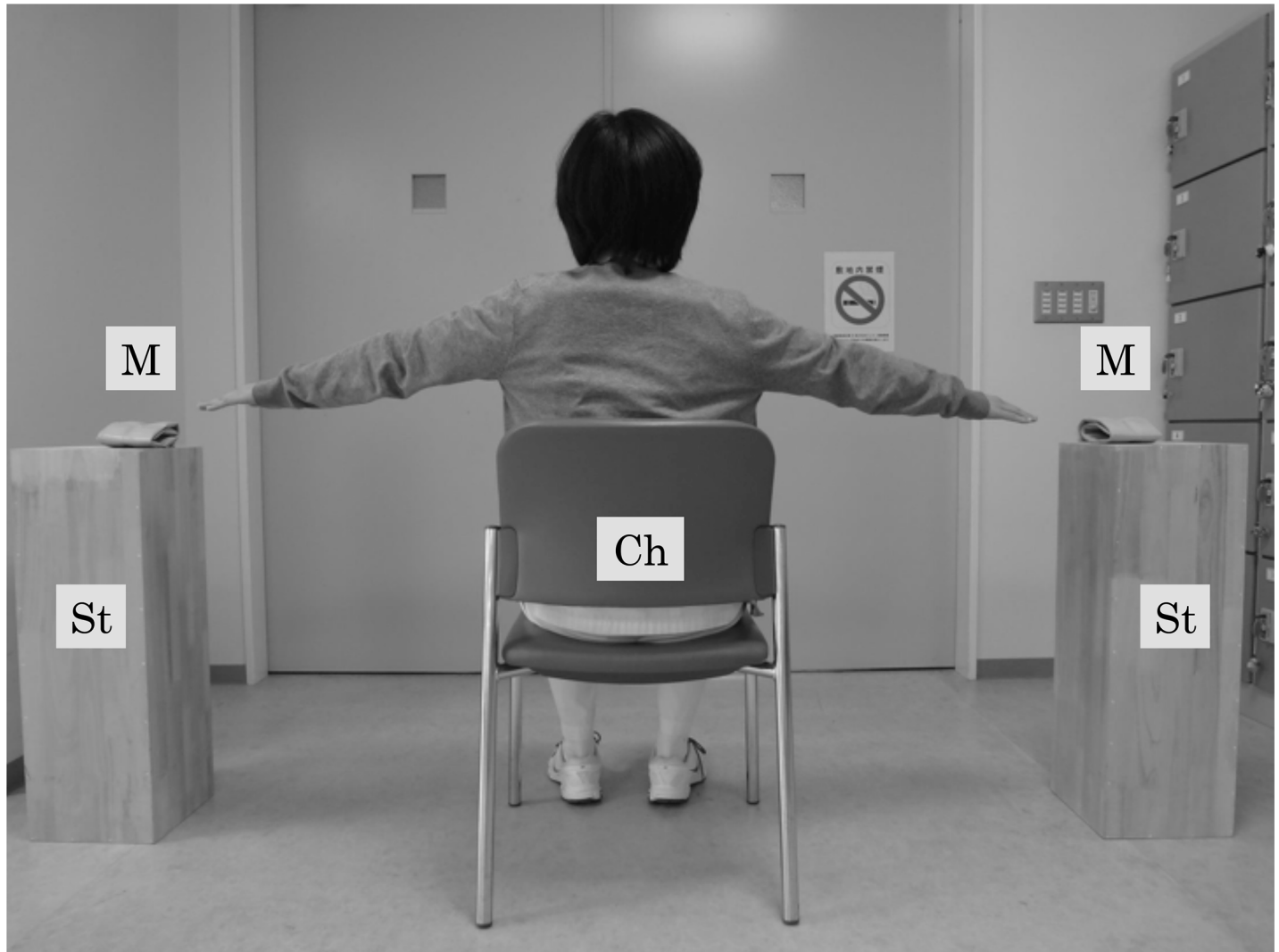
Fig 2. Measurement apparatus used in seated side tapping training. M: marker (diameter, 10 cm), St: stand (height, 72 cm), Ch: chair (height, 41 cm from a floor).
