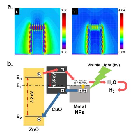
**Figure 4.** (a) FDTD simulation for showing generated surface plasmon enhancement from (i) silver and (ii) gold nanoparticles on the ZnO/CuO hetero nanostructure at the wavelength of 532 nm; (b) A schematic diagram of the theoretical bandgap structure at equilibrium state of the ZnO/CuO/M hierarchical nanostructure.
