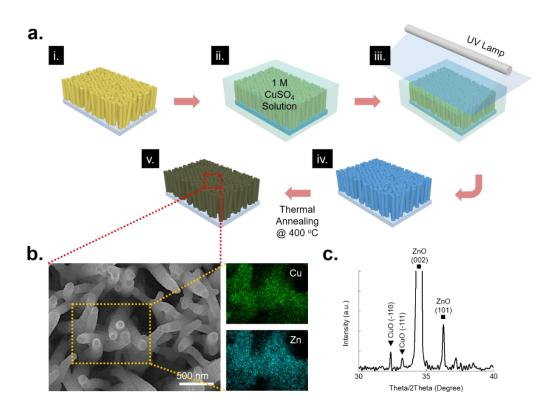
**Figure 1.** (a) A schematic of the fabrication process for ZnO/CuO hetero nanostructure; (b) Surface morphology of the ZnO/CuO hetero nanostructure and EDX component mapping images of Cu and Zn; (c) XRD spectra analysis of the ZnO/CuO hetero nanostructure, showing specific peaks of CuO and ZnO.
