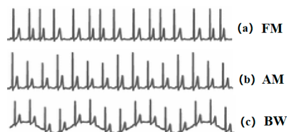
Figure 1. (a) Respiratory Sinus Arrhythmia (RSA) induced frequency modulation (FM). (b) Electrical axis rotation caused amplitude modulation (AM). (c) Baseline wander (BW) caused by chest movement.
