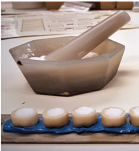
Figure 3. Potassium hydrogen difluoride crushed in a mortar and filled in crowns before melt-etching.
