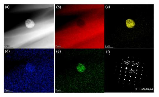
TEM elemental map results demonstrate that La-rich particles ( $Al_6Cu_6La$ ) form when La addition reaches 0.08%, as shown in Figure 4.
