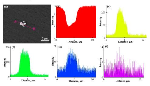
**Figure 3.** SEM image and EDS line-scanning results for Al-2Cu alloy inoculated with 0.4% Al-5Ti-1B + 0.08% La. (**a**) back-scattered electron image; (**b**–**f**) distributions of Al, Cu, La, Ti, and B along line A and B.
