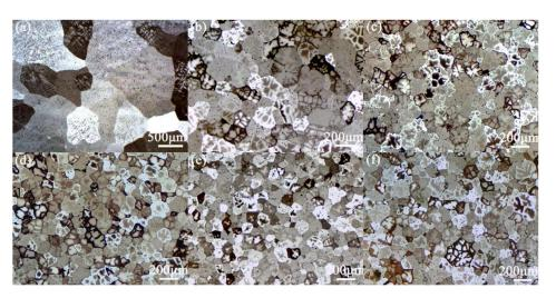
**Figure 1.** Microstructures of Al-2Cu alloy (**a**) without addition of inoculant and by adding 0.4% Al-5Ti-1B + La addition of (**b**) 0%, (**c**) 0.02%, (**d**) 0.06%, (**e**) 0.08%, and (**f**) 0.10%.
