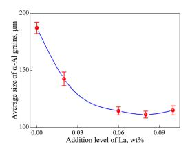
**Figure 2.** Average size of  $\alpha$ -Al grains in Al-2Cu alloy by adding 0.4% Al-5Ti-1B vs. La addition level.
