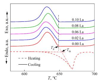
**Figure 5.** DTA heating and cooling curves for Al-2Cu alloy inoculated with 0.4% Al-5Ti-1B vs. La addition level.  $T_n$  and  $T_m$  are respectively the nucleation temperature and melting temperature. Heating/cooling rate is 10 K/min.
