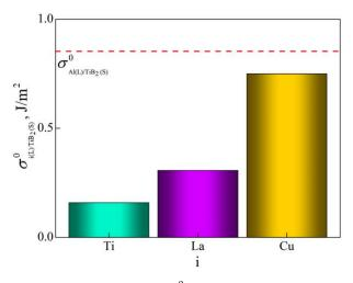
**Figure 6.** Interfacial energy  $\sigma_{i(L)/TiB_2(S)}^0$  of  $i(L)/TiB_2(S)$  at 660 °C.
