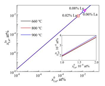
**Figure 7.**  $x_{La}^{In}$  as a function of  $x_{La}^{0}$ . Symbols present the points corresponding to the La addition level to melt.
