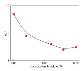
**Figure 8.** Calculated contact angle  $\theta$  varied with trace La addition level.
