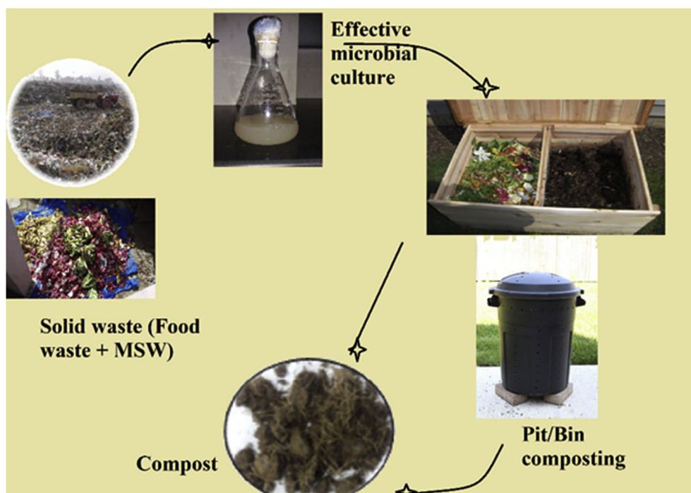
Figure 3. EM aided MSW Composting Operation.
