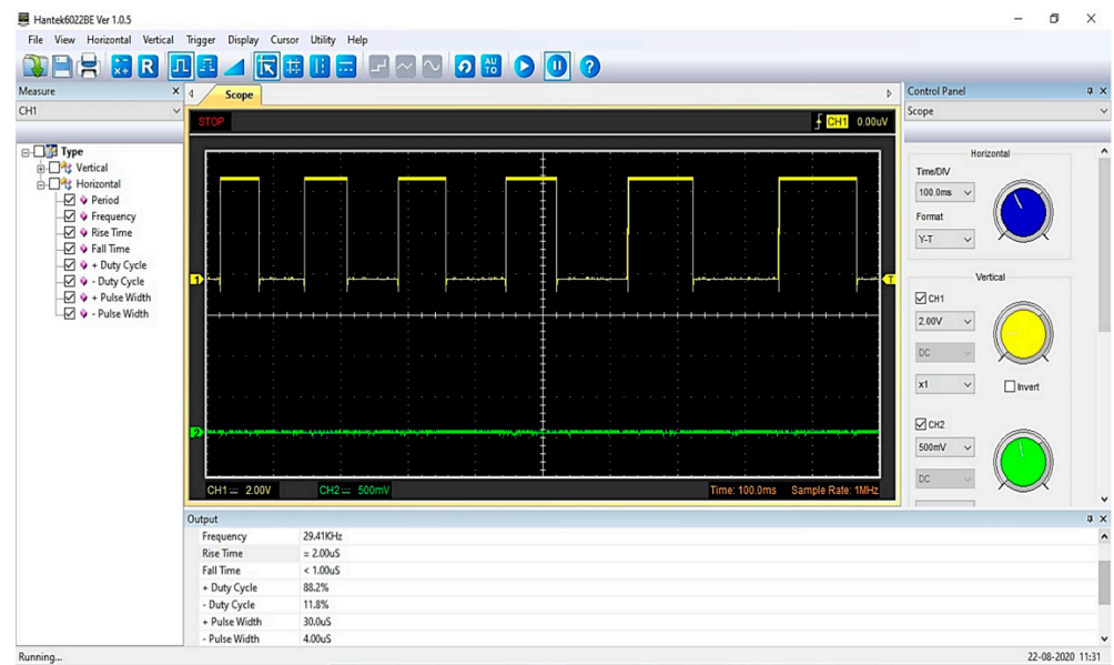
Figure 8. Image of waveform frequency on the user interface of the USB digital oscilloscope.
