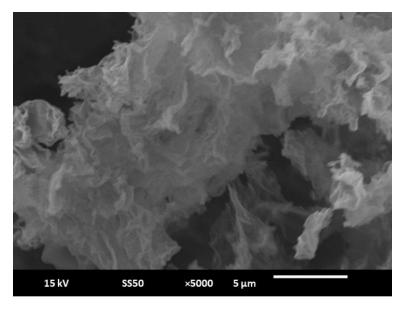
Figure 2. SEM image of RGO (scale: 5 µm).
