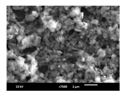
**Figure 6.** SEM image of  $MoS_2$  nanosheets (scale: 2  $\mu$ m).
