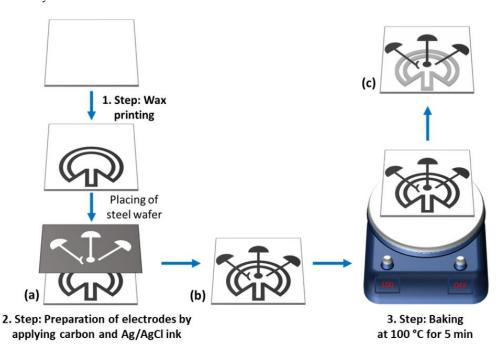
Scheme 1. Preparation of a paper electrode.
