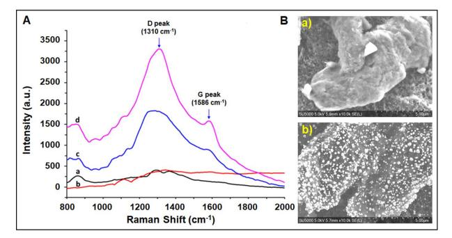
**Figure 1.** (**A**) Raman spectra of (a) nitrocellulose membrane (black), (b) carbon paste (red), (c) RGO-modified paper electrode (blue), (d) RGO-modified paper electrode after AuNP deposition (pink); (**B**) SEM images of (**a**) RGO and (**b**) AuNP/RGO-modified paper electrodes (scale: 5  $\mu$ m). Gold deposition was performed with the chronoamperometric technique in aqueous solution of the HAuCl<sub>4</sub> gold precursor by applying -0.3 V for 10 min.
