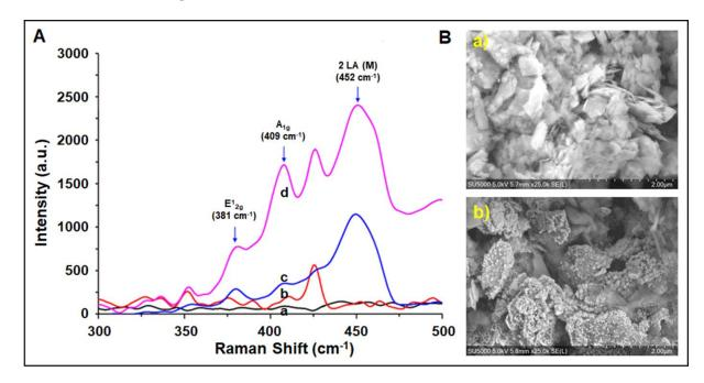
**Figure 5.** (**A**) Raman spectra of paper electrode: (a) nitrocellulose membrane (black), (b) carbon paste (red), (c) MoS<sub>2</sub>-modified paper electrode after AuNP deposition (red). (**B**) SEM images of (**a**) MoS<sub>2</sub>-nanosheet-modified paper electrode and (**b**) MoS<sub>2</sub>-modified paper electrode after gold electrodeposition (scale: 2 μm).
