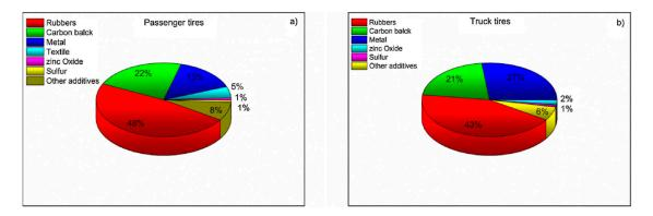
**Figure 2.** Tire composition for passenger cars (left) and trucks (right). Reproduced with permission from: [14].
