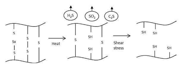
**Figure 4.** Mechanism for the cross-linking breakage in a thermomechanical devulcanization process. Reproduced with permission from [14].
