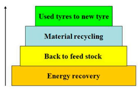
Figure 7. Proper waste management hierarchy. Reproduced with permission from [21].
