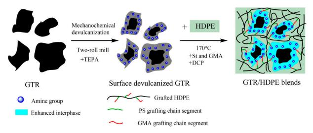
**Figure 6.** Schematic illustration of the preparation of ground truck-tire rubber/high-density polyethylene (GTR/HDPE) blend by combining surface devulcanization and in situ grafting technology (styrene (St), glycidyl methacrylate (GMA), and dicumyl peroxide (DCP) were used). Reproduced with permission from [15].
