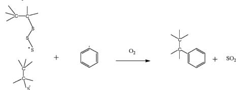
Figure 5. Plausible reaction mechanism of devulcanization. Reproduced with permission from [39].
