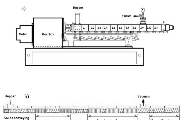
**Figure 3.** A twin-screw extruder for continuous devulcanization. Reproduced with permission from [18], (a) Shows a scheme of the extruder. (b) is a typical screw configuration with the different process sections.
