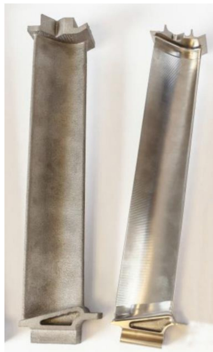
Figure 4. Comparison of turbine blades manufactured by EBM before and after conventional machining © 2018, Avio Aero [32].
