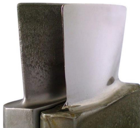
Figure 6. Surface finish after rough machining (left) and finish machining (right) [34] © EMAG GmbH & Co. KG, 2021.
