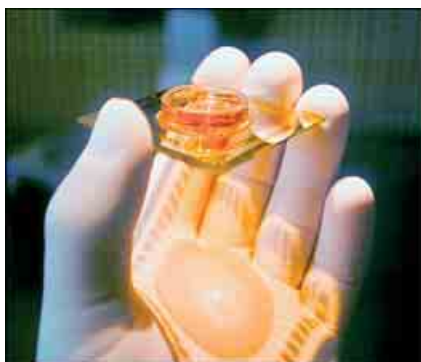
Figure 2. MEART's brain (above) and a MEA culture dish (below). A week-old culture of ~50 000 neurons and glia from embryonic rat cortex, growing in a MEA and forming a dense network 1–2 mm across. Fifty-nine 30 \mu\text{m} electrodes spaced at 200 \mu\text{m} intervals connect a few hundred of the network's neurons to the outside world, by allowing their activity to be extracellularly recorded or evoked by electrical stimulation.
