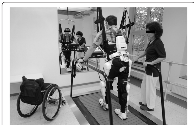
Fig. 1 Hybrid assistive limb ® (HAL ® ). Bodyweight supported treadmill training with the HAL ® exoskeleton. (Copyright V. Daum, Bergmannsheil Bochum)
