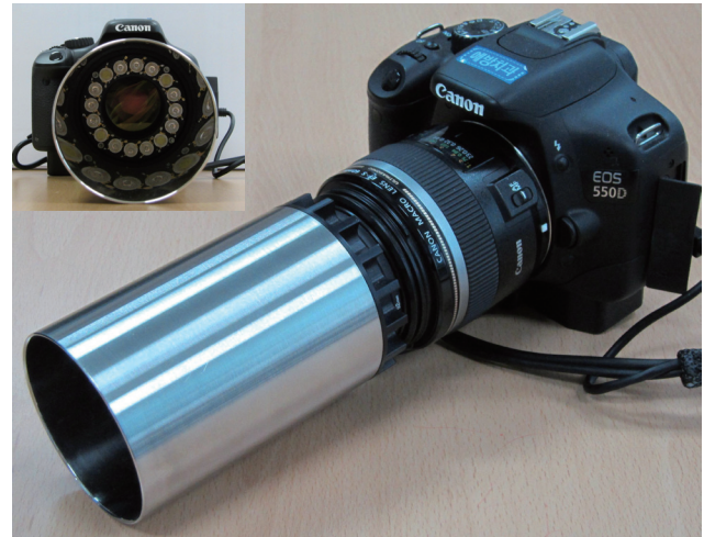
Figure 1. The QLF device is based on a DSLR camera equipped with an illumination tube with white and blue light-emitting diodes positioned in a ring around the lens opening. QLF, quantitative light-induced fluorescence; DSLR, digital single lens reflex.
