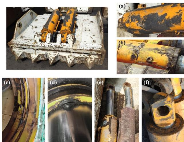
**Figure 1.** Different failure types of the tail beam jack: (a) surface wear, (b) weld crack, (c) seal breakage, (d) hydraulic oil leak, (e) piston rod bend, and (f) deformation of hinge hole.
