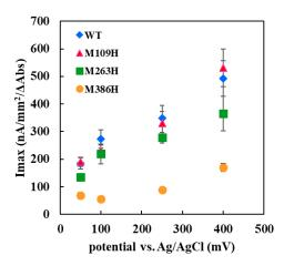
**Figure 4.** Imax value dependency on the applied potential vs. Ag/AgCl for the electrode immobilized with WT, Met109His, Met263His, or Met386His enzyme.
