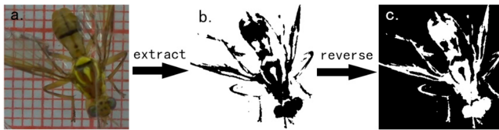
Figure 3. The extraction process of body part information of Bactrocera minax . (a) The original video frame contains the Bactrocera minax and the background which is RGB image; (b) Image P_b only contains background, the gray value of the black region is 0, and the gray value of the white region is 255; (c) Image P_b after reversal.
