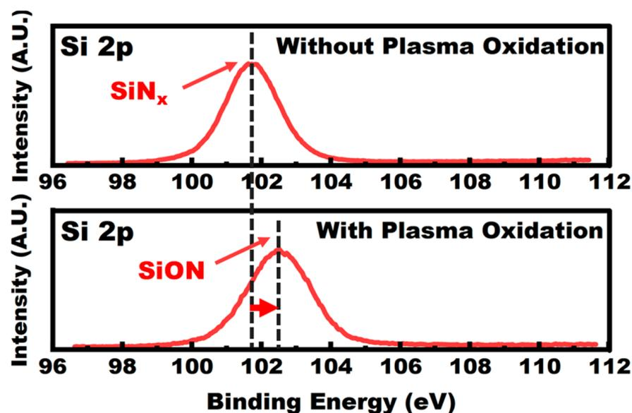
Figure 3. Si2p XPS results on the surface  $\text{SiN}_x$  film without and with plasma oxidation.
