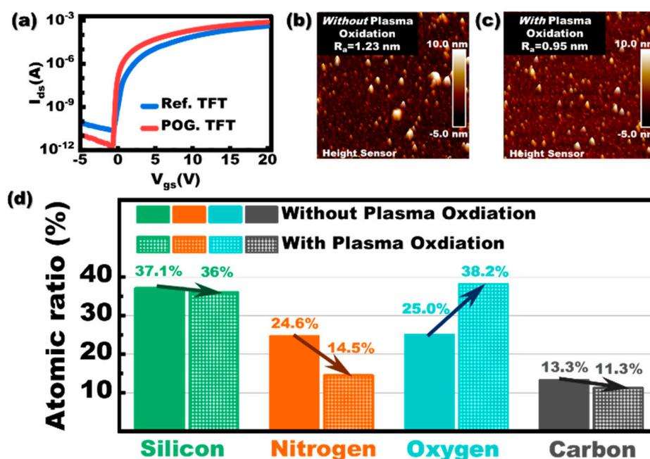
Figure 2. (a) Transfer characteristic curves for Ref. TFT and POG. TFT. The surface morphology for SiN<sub>x</sub> (b) without plasma oxidation and (c) with plasma oxidation. (d) The atomic ratio for the surface of SiN<sub>x</sub> thin film without/with plasma oxidation.
