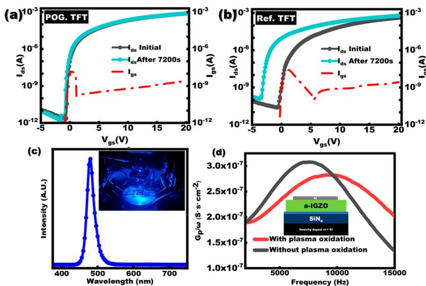
Figure 5. The curves of transfer characteristic before/after NBIS test for (a) Ref. TFT and (b) POG. TFT; (c) spectrum of blue LED used in NBIS test; (d)  $G_p/\omega$  as the function of frequency for Ref. and POG. MOS capacitor.
