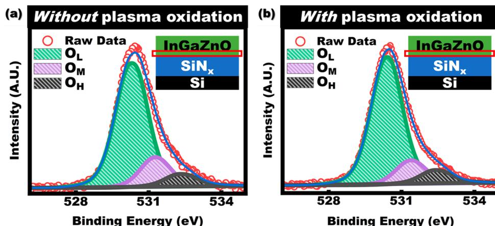
Figure 4. XPS results for surface of SiN<sub>x</sub> thin film (a) without (b) with plasma oxidation.
