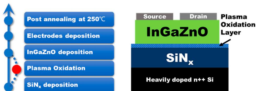
Figure 1. Process flow diagram and structure of InGaZnO TFT in this work.
