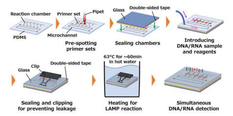
**Figure 3.** Operating procedure for the multiplex loop-mediated isothermal amplification (LAMP) assay employed in microfluidic diagnostic devices for the simultaneous detection of DNA- and RNA-based plant viruses.
