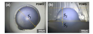
**Figure 5.** Optical microscopy images showing (a) close-up plane and (b) cross-sectional views of a PDMS reaction chamber precisely replicated from a hemispherical polymer bead glued on the SU-8 pattern.
