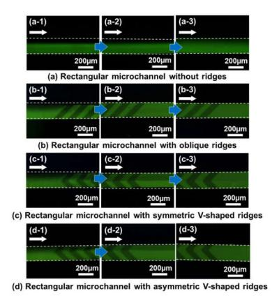
Figure 8. Experimental results showing fluorescence microscopy images (taken with an optical filter B-2A, gain:  $1\times$ , exposure time: 2 s) of the mixing process in (a) a rectangular microchannel without ridges, and (b) a chaotic mixer with oblique ridges, (c) symmetric V-shaped ridges, and (d) asymmetric V-shaped ridges. Fluorescein-dyed water (1 mM) and pure water were introduced at the same flow rate of  $5 \,\mu$ L/min.
