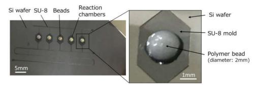
**Figure 4.** Photographs of an SU-8 master mold pattern on an Si wafer, in which hemispherical polymer beads (2 mm in diameter) were bonded with epoxy adhesive on the surface of five microchamber patterns to create deep localized structures, after replicating this mold in PDMS.
