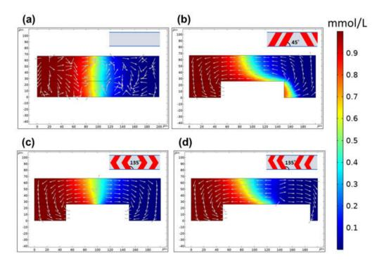
**Figure 11.** The concentration distribution (contour) and transverse velocity fields (arrows) across the microchannel cross-section at the position y = 0.45 mm away from the inlet. (a) Rectangular microchannel without ridges. (b) Chaotic mixer with oblique ridges, (c) symmetric V-shaped ridges, and (d) asymmetric V-shaped ridges.
