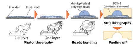
**Figure 2.** Fabrication process for a PDMS-based microfluidic diagnostic device fabricated by a modified soft-lithography process assisted with hemispherical polymer beads to create deep localized microchamber structures.
