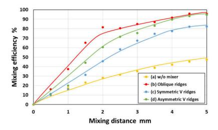
**Figure 12.** Simulation results showing the mixing efficiency of three different chaotic mixers with periodic oblique, symmetric V-shaped, and asymmetric V-shaped ridges as a function of the mixing distance along the flow direction. For comparison, the data obtained in a rectangular microchannel without ridges is also plotted in the graph.
