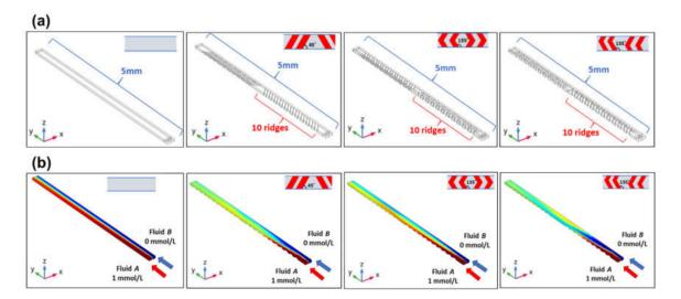
Figure 10. (a) Three-dimensional FEM models showing a rectangular microchannel without any ridge structures, and with periodic oblique ridges, symmetric V-shaped ridges, and asymmetric V-shaped ridges. (b) Simulation results showing the concentration contours of two different fluids (with a concentration of 0 and 1 mmol/L) in each microchannel at a flow velocity of 0.0128 m/s each (equivalent to  $5 \mu L/min$ ).
