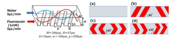
**Figure 7.** Schematic diagram of chaotic mixing (illustrated by the streamlines of two fluids) in a microchannel and designs of three types of chaotic mixers. The mixing efficiency was estimated in (a) a rectangular microchannel without ridges, which was used for comparison, and (b) a chaotic mixer with periodic oblique, (c) symmetric V-shaped, and (d) asymmetric V-shaped ridges embedded in the microchannel.
