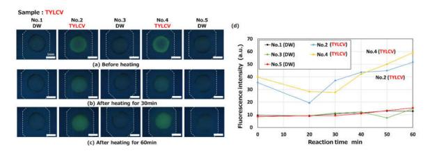
**Figure 14.** Fluorescence microscopy images showing the LAMP detection of a DNA-based plant virus (tomato yellow leaf curl virus, TYLCV) observed (a) before heating and after heating for (b) 30 min and (c) 60 min at 63 °C (taken with an optical filter BV-2A, gain: 1×, exposure time: 2 s). A primer set for the detection of TYLCV was pre-spotted in reaction chambers (Nos. 2 and 4). (d) Changes in fluorescence intensities as a function of the reaction time.
