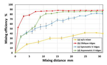
**Figure 9.** Experimental results showing the mixing efficiency of three different types of chaotic mixers with periodic oblique, symmetric V-shaped, and asymmetric V-shaped ridges as a function of the mixing distance along the flow direction. For comparison, the data obtained in a rectangular microchannel without ridges is also plotted in the graph. Note that each point and error bar in the plot represent the mean values and their standard deviations, respectively.
