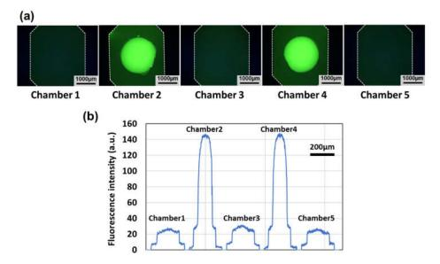
**Figure 6.** A comparison of the fluorescence intensity of two kinds of microchambers replicated with or without a hemispherical polymer bead. (a) Fluorescent microscopy images of microchambers (gain: 1×, exposure time: 2 s). (b) Cross-sectional profiles of the fluorescence intensity across the center of each microchamber.
