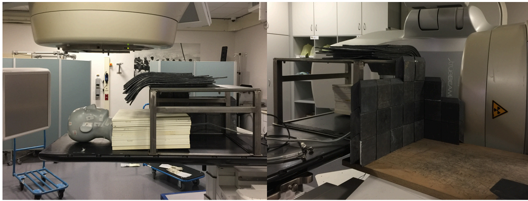
Fig. 3. Phantom set-up for fetal dose estimation during the VMAT photon treatment.
