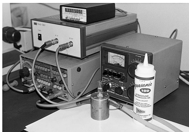
Fig. 2. General view of ultrasonic generator. Monitor, amplifier and function generator from upper left; output meter and gel for adhesion on the right; and glass cell containing experimental solution in the center.
