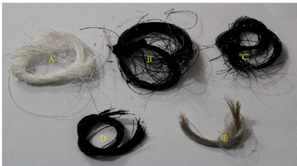
Figure 2. The aspect of the composite nanoparticles–polymer membranes ( Os_{np} -PM): A —polypropylene hollow fiber membranes support (PP); B —Os-PPM i from OsO_4 - i -propanol-10-undecenoic acid; C —Os-PPM t from OsO_4 - t -butanol-10-undecenoic acid; D —Os-PPM n from OsO_4 - n -decanol-10-undecenoic acid; E —Os-PPM p from OsO_4 -pure 10-undecenoic acid.
