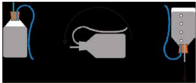
Figure 2: Device producing constant flow rate to calibrate a flowmeter. The vent maintains constant pressure at the level of the bung and hence constant flow rate through the outlet tube
