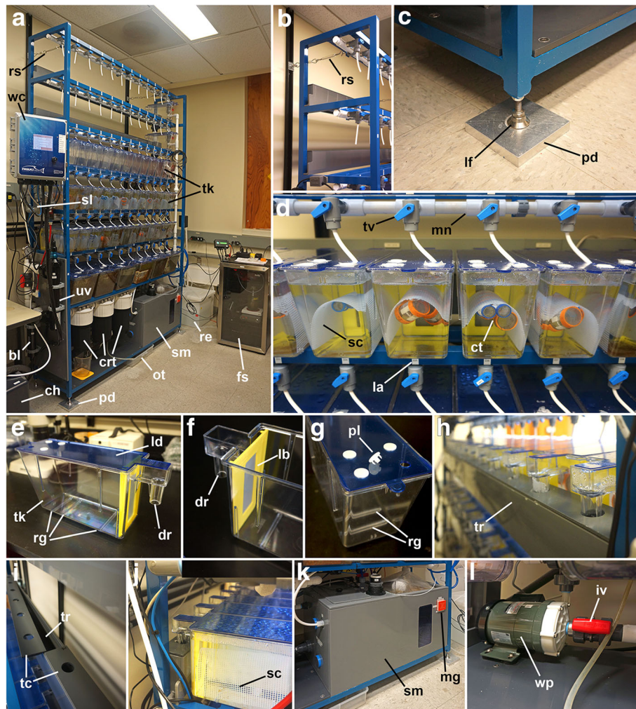
Fig. 1 a–l Overview of the rack system, individual tanks, drain trough, and water pump. a Rack system to the left and associated feeding system to the right. Part of the external chiller can be seen on the floor in the bottom, far left corner. b Detail of the wall restraints that prevent tipping. c Detail of the foot pad to prevent sliding and to distribute weight (see Additional file 3A). d Row of 3-l tanks showing the manifold and valves that supply water to these tanks. Some culture tubes are seen inside these tanks, which are held down by the curved plastic mesh. e Empty 3-l tank with lid. f Detail of the overflow drain and larval baffle. g Detail of the plastic plugs used to cap unused holes in the lid. h Drain trough that receives the tanks' overflow drain tubes. i Detail of the PVC covers for the drain troughs (see Additional file 3B–C). j Another view of the curved plastic restraining screen. k Sump. l Main water pump. This pump is secured to the bottom PVC deck with four bolts and rubber shock mounts. bl, ballast; ch, chiller; crt, cartridge filters; ct, culture tubes; dr, overflow drain; fs, feeding system; iv, water pump intake valve; la, labels; lb, larval baffles; ld, tank lid; lf, leveling feet; mg, magnet; mn, manifold; ot, overflow tray; pd, foot pad; pl, plugs; re, reservoirs; rg, plastic ridges; rs, rack restraint; sc, plastic restraining screen; sl, sensor side loop; sm, sump; tc, trough covers; tk, tanks; tr, drain trough; tv, tank valve; uv, UV lamp; wc, Walchem 900 controller; wp, water pump
