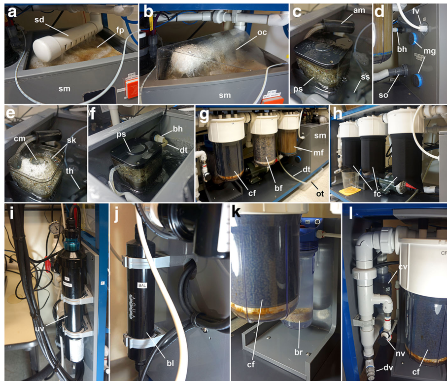
Fig. 3 a–l Overview of the water filtration system. a Slotted drain diverter returning water to the right compartment of the sump through the coarse filter pad (origami cover has been removed). b View with the origami cover installed over the slotted drain diverter and large sump opening (see Additional file 3D). c Detail of the protein skimmer located in the left compartment of the sump. Small plastic sump lid has been removed to reveal the protein skimmer. The air muffer prevents water from entering the airline to the skimmer. Part of the perforated skimmer stand can be seen that supports the skimmer at the correct height. d Detail of the left side of the sump showing two magnets that hold the skimmer in place. The bulkhead compression fitting is also seen, through which the skimmer cup drain tubing passes to exit the sump. e View of the skimmer cup with its cover removed to show the chimney and the foamy skimmate, rich with organic materials. The titanium heater is also seen crossing the floor of the sump. f Another view of the protein skimmer. The skimmer cup drain tube is seen passing to the bulkhead compression fitting. g View of the three large canister filters. The skimmer cup drain tubing is seen passing to an overflow collecting tray located on the floor under the rack system. h Opaque black elastic covers for the canister filters, which are used to prevent algal growth. i UV lamp. j Ballast for the UV lamp. k View of the bioreactor located just behind the activated carbon filter. This filter canister is anchored by a PVC stand, and a small amount of the PHA pellets can be seen at the bottom of the filter bowl. This filter also has an opaque black elastic cover, which has been removed for this photo. l View of the small needle valve that controls water flow to the bioreactor to keep the PHA pellets in motion. The main system drain and the large one-way check valve are also seen. The latter prevents water from traveling backwards through the filters during a feeding cycle. am, air intake muffer; bf, biological filter; bh, bulkhead compression fitting; bl, ballast; br, bioreactor; cf, activated carbon filter; cm, chimney; cv, reverse flow check valve; dt, drain tubing; dv, main drain valve; fc, opaque filter covers; fp, coarse filter pad; fv, filler valve; mg, magnets; mf, fine mechanical filter; nv, needle valve; oc, origami cover; ps, protein skimmer; sd, slotted drain diverter; sk, skimmate; so, sump outlet; ss, skimmer stand; th, titanium heater. Other labels are the same as those used in Fig. 1
