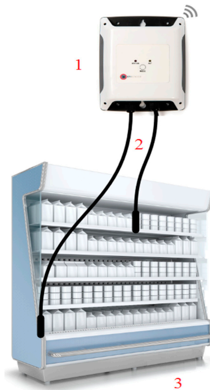
Figure 1. The SLR-DS18B20 System Architecture. This diagram depicts the proposed system’s architecture. The Raspberry Pi Zero W (Device 1) is connected to the series of DS18B20 sensors (the sensors are given the number 2) using pins 7, 17, and 25. Pin 7 is responsible for the communication, pin 17 provides 3.3 voltage to the device, while pin 25 is responsible for grounding the circuit. Then, these sensors are inserted into a commercial fridge (device 3).
