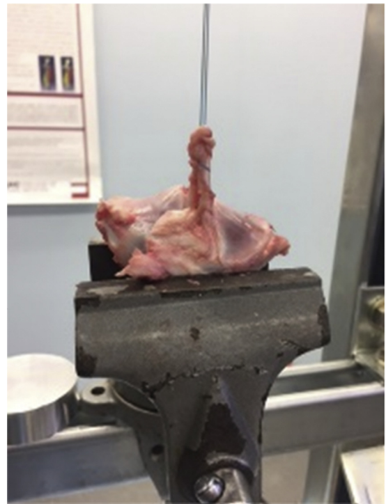
Fig 1. Test setup of porcine tibia with simulated anterior cruciate ligament tear captured with Krackow locking suture.
