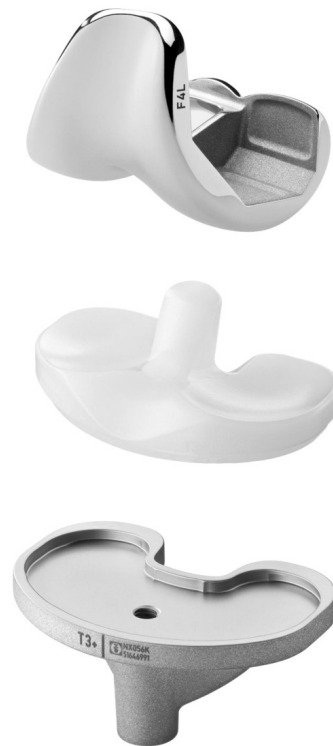
Fig. 1. The photographs show the Vega-PS prosthesis. The anterior and posterior narrowing of the femoral component with a low profile intercondylar box minimizes interference with the surrounding soft tissues. Fifty-five degrees posterior inclination of the post acts to avoid post-edge loading for better load distribution, prevents impingement with the extensor mechanism, and increases resistance to dislocation. The deepened anterior cutout of the insert allows smooth articulation with the patellar tendon.
