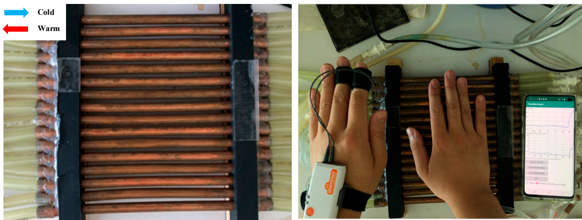
Figure 5. Thermal grill (left) and an example of data collection (right).
