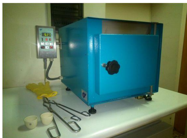
Figure 2. Muffle furnace for the incineration of samples.
