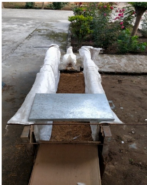
Fig. 2. Setup for the run-away test along with entry and exit for birds and not influenced by the surrounding environment.
