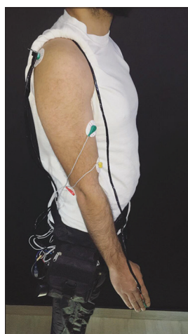
Figure 2: Prototype attached to the human body. The bag is strapped to the thigh and waist. Heart rate and oxygen saturation sensor are attached to the forefinger. Electromyography electrodes are placed over the biceps muscle, and an accelerometer is located on the back or around the chest
