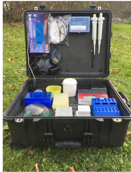
Fig. 1. Diagnostics-in-a-Suitcase. It contains all equipment and reagents for performing the RT-RPA assay.
