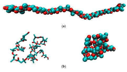
**Figure 14.** The initial configuration of the PHBV (**a**) (radius of gyration  $R_g = 8.8$  nm) and after 1 ns simulation in vacuum (**b**).
