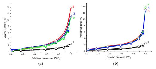
**Figure 7.** Water vapor adsorption (filled symbols) and desorption (open symbols) isotherms at 25 °C on the samples: 1—PHBV/PCL(1:1), 2—PHBV/PCL(1:1)/CNC(PVP)–5, 3—PHBV/PCL(1:1)/CNC(PVP)–10, 4—PHBV/PCL(1:1)/CNC(PVP)–15 (**a**); 5—PHBV/PCL(1:1)/CNC(PAM)–5, 6—PHBV/PCL(1:1)/CNC(PAM)–10, 7—PHBV/PCL(1:1)/CNC(PAM)–15 (**b**).
