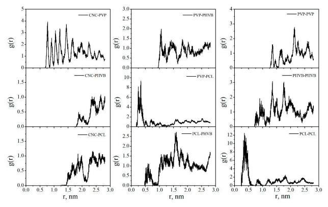
**Figure 28.** The radial distribution functions between the centers of mass of the composite components in vacuum.
