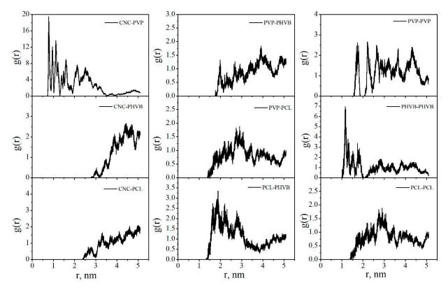
**Figure 29.** The radial distribution functions between the centers of mass of the composite components in DCM.
