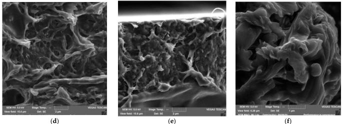
**Figure 3.** SEM images of the surface (**a**–**c**) and cleavage (**d**–**f**) of the PHBV/PCL/CNC composite films: PHBV/PCL(1:1)/CNC(PAM)–5 (**a**,**d**); PHBV/PCL(1:1)/CNC(PAM)–10 (**b**,**e**); PHBV/PCL(1:1)/CNC(PAM)–15 (**c**,**f**). The scale is 2 µm (**a**,**b**,**d**,**e**); 1 µm (**c**,**f**).
