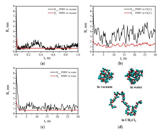
**Figure 15.** Time dependences of the end-to-end distance  $(R_{e-t-e})$  and radius of gyration  $(R_g)$  of the PHBV in vacuum (**a**), DCM (**b**), and water (**c**); instant snapshots of the PHBV chain conformations in vacuum, DCM, and water (**d**).
