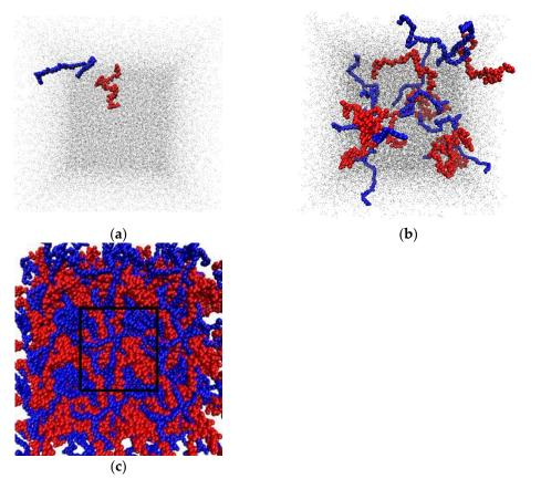
**Figure 21.** Snapshots of the systems under study at the end of the simulation: System 1 (**a**); System 2 (**b**); System 3 (**c**). PCL is shown in blue, PHBV in red, and DCM in grey.
