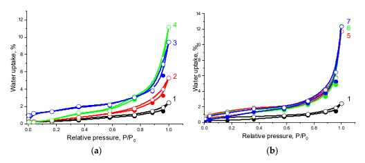
**Figure 8.** Water vapor adsorption (filled symbols) and desorption (open symbols) isotherms at 25 °C on the samples: 1—PHBV/PCL(1:2), 2—PHBV/PCL(1:2)/CNC(PVP)–5, 3—PHBV/PCL(1:2)/CNC(PVP)–10, 4—PHBV/PCL(1:2)/CNC(PVP)–15 (**a**); 5—PHBV/PCL(1:2)/CNC(PAM)–5, 6—PHBV/PCL(1:2)/CNC(PAM)–10, 7—PHBV/PCL(1:2)/CNC(PAM)–15 (**b**).
