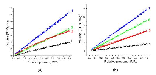
**Figure 6.** Low-temperature nitrogen adsorption (filled symbols) and desorption (open symbols) isotherms on the samples: 1—PHBV/PCL(1:2), 2—PHBV/PCL(1:2)/CNC(PVP)–5, 3—PHBV/PCL(1:2)/CNC(PVP)–10, 4—PHBV/PCL(1:2)/CNC(PVP)–15 (**a**); 5—PHBV/PCL(1:2)/CNC(PAM)–5, 6—PHBV/PCL(1:2)/CNC(PAM)–10, 7—PHBV/PCL(1:2)/CNC(PAM)–15 (**b**).
