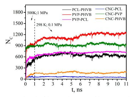
**Figure 23.** The number of close contacts between atoms of the components within a distance of 0.5 nm.
