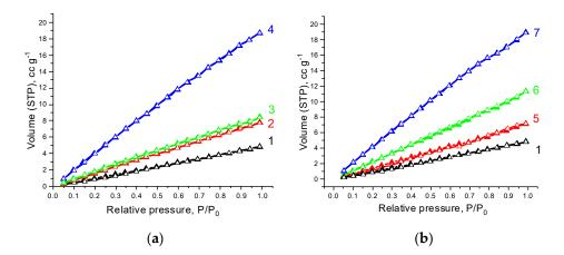
**Figure 5.** Low-temperature nitrogen adsorption (filled symbols) and desorption (open symbols) isotherms on the samples: 1—PHBV/PCL(1:1), 2—PHBV/PCL(1:1)/CNC(PVP)–5, 3—PHBV/PCL(1:1)/CNC(PVP)–10, 4—PHBV/PCL(1:1)/CNC(PVP)–15 (**a**); 5—PHBV/PCL(1:1)/CNC(PAM)–5, 6—PHBV/PCL(1:1)/CNC(PAM)–10, 7—PHBV/PCL(1:1)/CNC(PAM)–15 (**b**).
