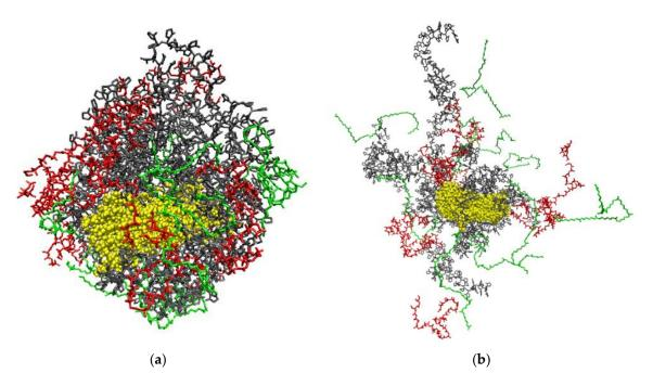
**Figure 26.** Snapshot of the initial (**a**) and final (**b**) configuration of the PHVB/PCL/PVP/CNC composite in DCM: PVP is colored grey; CNC is colored yellow; PHBV is colored red; PCL is colored green. DCM molecules are not depicted for clarity.
