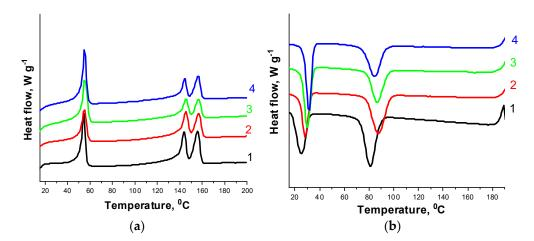
**Figure 10.** DSC curves for the PHBV/PCL(1:1) mixture (1); PHBV/PCL(1:1)/CNC(PVP)–5 (2), PHBV/PCL(1:1)/CNC(PVP)–10 (3), and PHBV/PCL(1:1)/CNC(PVP)–15 (4) composites: at heating (**a**); at cooling (**b**).
