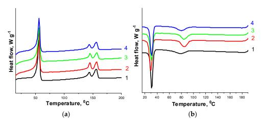
**Figure 11.** DSC curves for the PHBV/PCL(1:2) mixture (1); PHBV/PCL(1:2)/CNC(PVP)–5 (2), PHBV/PCL(1:2)/CNC(PVP)–10 (3), and PHBV/PCL(1:2)/CNC(PVP)–15 (4) composites: at heating (a); at cooling (b).
