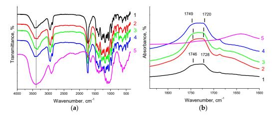
**Figure 9.** FTIR spectra of the PHBV/PLC(1:1) mixture (1); PHBV/PCL(1:1)/CNC(PVP)–5 (2), PHBV/PCL(1:1)/CNC(PVP)–10 (3), PHBV/PCL(1:1)/CNC(PVP)–15 (4) composites; the neat CNC (5): (a) in the 4000–400 cm<sup>-1</sup> range; (b) in the 1850–1600 cm<sup>-1</sup> range.
