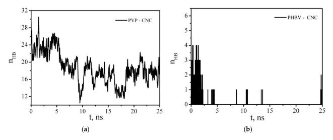
Figure 19. Time dependence of the number of PVP–CNC (a) and PHBV–CNC (b) hydrogen bonds.
