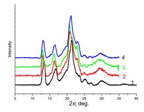
**Figure 13.** X-ray diffraction patterns of the PHBV/PCL(1:1) mixture (1); PHBV/PCL(1:1)/CNC(PVP)– 5 (2), PHBV/PCL(1:1)/CNC(PVP)–10 (3), and PHBV/PCL(1:1)/CNC(PVP)–15 (4) composites.
