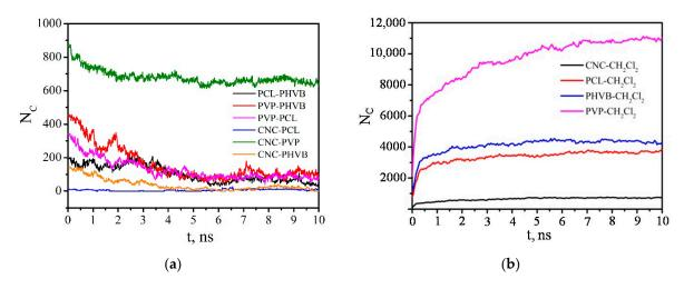
**Figure 27.** The time dependence of the number of close contacts between any pair of atoms of CNC–polymer, polymer–polymer (**a**), and CNC-DCM, polymer–DCM (**b**).
