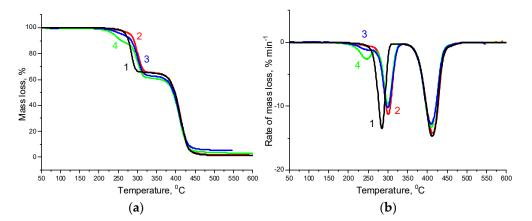
**Figure 12.** TG (**a**) and DTG (**b**) curves for the PHBV/PCL(1:2) mixture (1); PHBV/PCL(1:2)/CNC(PVP)–5 (2), PHBV/PCL(1:2)/CNC(PVP)–10 (3), and PHBV/PCL(1:2)/CNC(PVP)–15 (4) composites.
