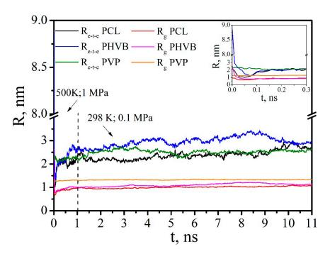
**Figure 24.** The time dependence of the end-to-end distance and radius of gyration for PCL, PHVB, and PVP.
