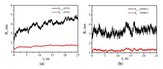
**Figure 17.** Time dependence of the end-to-end distance  $R_{e-t-e}$  and radius of gyration  $R_g$  of PVP (**a**) and PHBV (**b**).
