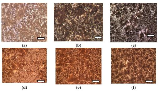
**Figure 4.** POM images of the surface of the PHBV/PCL/CNC composite films: PHBV/PCL(1:1)/CNC(PVP)–5 (**a**); PHBV/PCL(1:1)/CNC(PVP)–10 (**b**); PHBV/PCL(1:1)/CNC(PVP)–15 (**c**); PHBV/PCL(1:1)/CNC(PAM)–5 (**d**); PHBV/PCL(1:1)/CNC(PAM)–10 (**e**); PHBV/PCL(1:1)/CNC(PAM)–15 (**f**). The scale is 100 μm.
