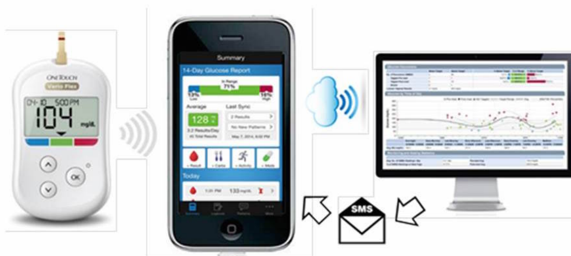
Figure 1. Study data flow. All participants used the OneTouch Verio Flex meter to conduct self-monitoring of blood glucose (SMBG). SMBG data were transmitted wirelessly from the meter to the smartphone containing the diabetes management app OneTouch Reveal. SMBG data were automatically uploaded via the cloud to a Web-based version of the app accessible by site health care professionals (HCPs) on their office computers. HCPs reviewed the 14-day app report for each participant to assist in formulating diabetes-related text messages sent to the participant's smartphone.
