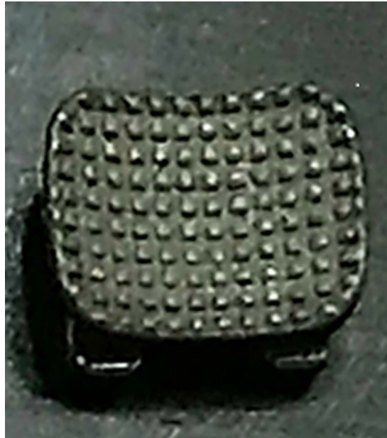
Figure 1. A metal bracket base with a mesh design containing numerous tiny undercuts to ensure maximum mechanical interlocking between the bracket and adhesive.
