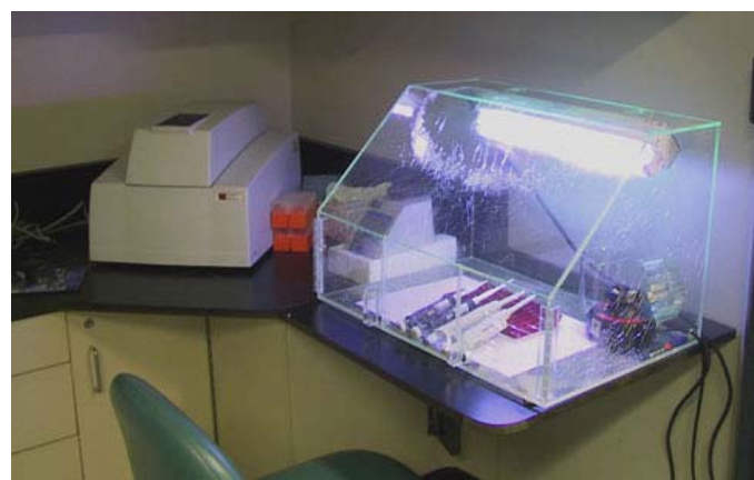
Fig. 6: UV-equipped Plexiglas hood is used in order to prevent sample contamination.
