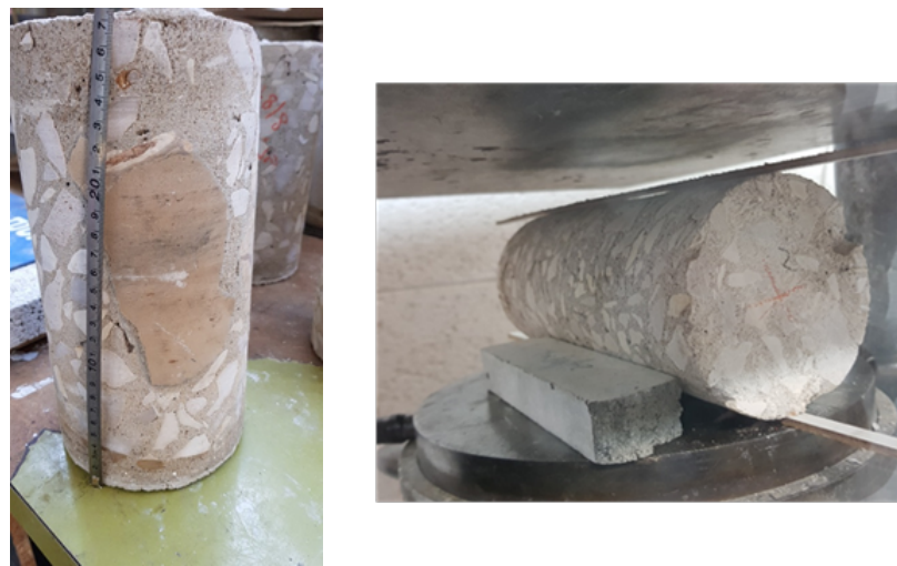
Figure 2. Cylindrical authentic LPC specimens.
