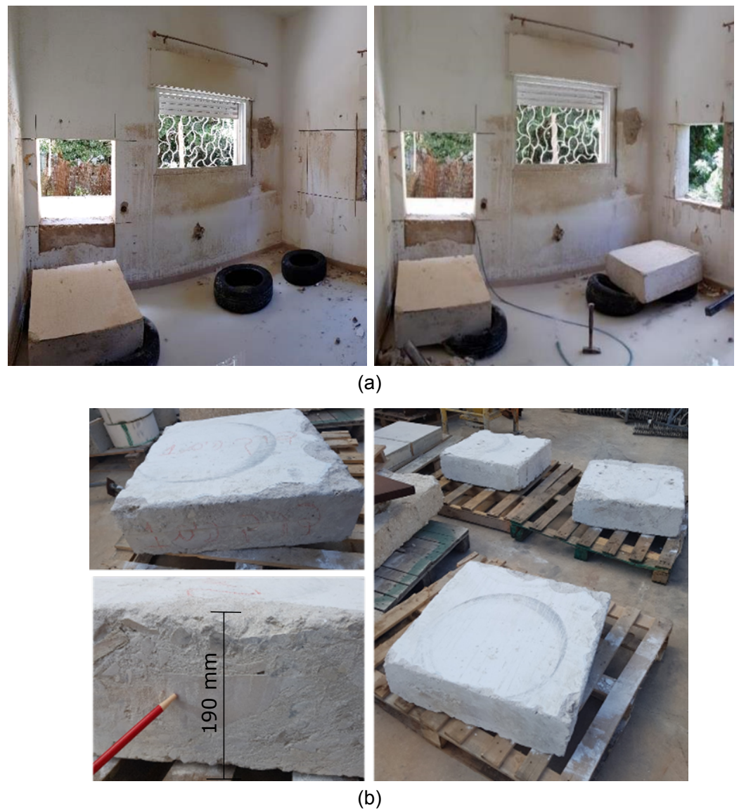
Figure 1. (a) Extraction of authentic specimens and (b) authentic specimens with large aggregates/stones.
