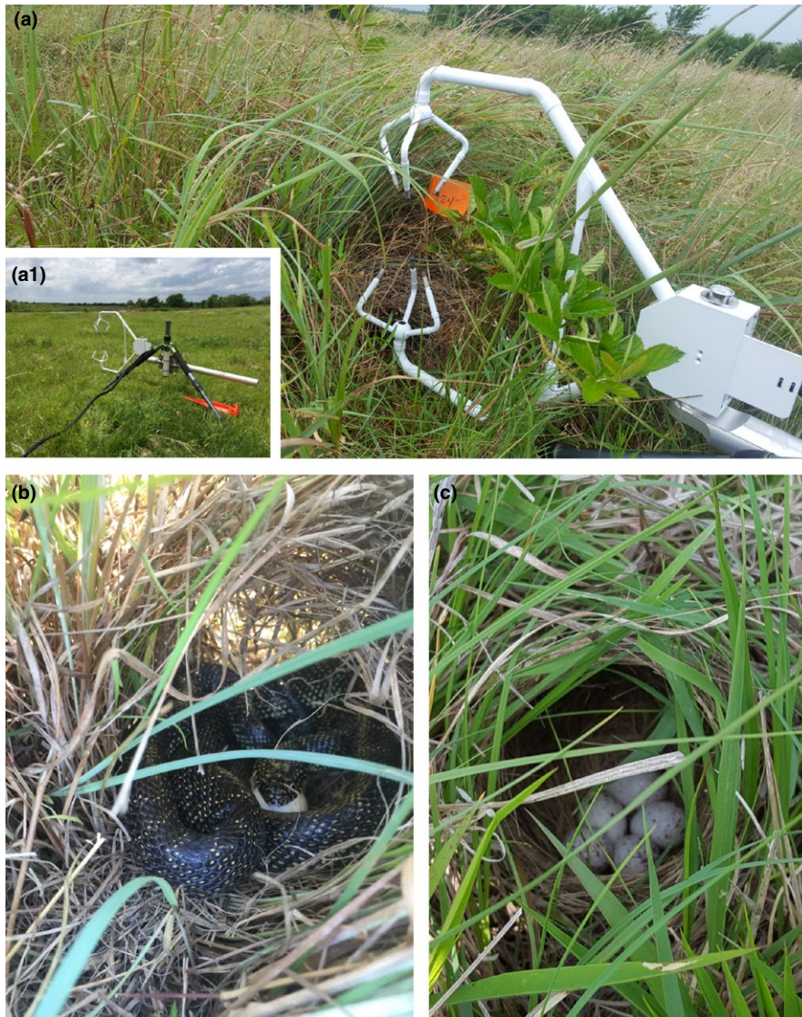
FIGURE 2 (a.1) Sonic anemometer mounted on a camera tri-pod (a) recording airflow velocity readings at a Northern Bobwhite nest. (b) A speckled kingsnake depredating a bobwhite nest and (c) a Eastern Meadowlark nest with a full clutch of eggs. All photographs were taken on the McFarlin-Ingersoll ranch, Inola, Oklahoma, USA, in 2015 and 2016. Photographs are courtesy of (a, a.1, c) D. Fogarty and (b) C. Fitzmorris
