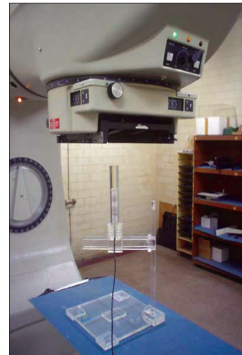
Figure 2: Photograph of mini phantom in the treatment position with Co-60 machine, which was fabricated for this study and used for dose measurement
