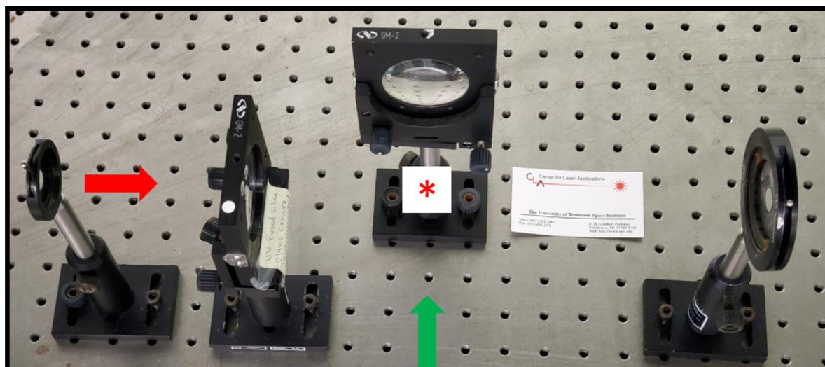
**Figure 1.** Module for recording shadowgraphs of optical breakdown in air. The collimated laser beam (red arrow) is focused with  $f/20$  optics. The asterisk symbolically indicates optical breakdown. The interaction area is illuminated by a time-delayed laser beam (green arrow), and images are projected onto a screen (not shown) and recorded with a digital camera.
