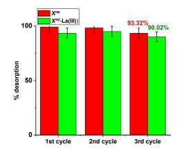
**Figure 16.** Desorption efficiency (%) for As(V) recovery using X<sup>np</sup> and X<sup>np</sup>-La(III) (As(V) concentration: 100 mg/dm<sup>3</sup>, desorbing agent: 1M NaOH, sorption/desorption time: 6 h, shaking speed 180 rpm, temperature 295 K).
