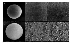
**Figure 2.** SEM images of X<sup>np</sup> before (**A**–**C**) and after the modification with La(III) ions (**D**–**F**) at various magnifications (250×; 2500× and 5000×).
