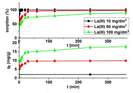
**Figure 7.** Lanthanum(III) sorption efficiency and sorption capacities as a function of time on  $X^{np}$  ( $c_0 = 10, 50$  and  $100 \text{ mg/dm}^3$ , pH = 4, shaking speed 180 rpm, temperature 295 K).
