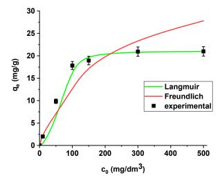
**Figure 9.** The Langmuir and Freundlich sorption isotherms of La(III) on X<sup>np</sup> (pH 4, shaking speed 180 rpm, temperature 295 K).
