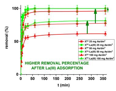
**Figure 12.** Arsenic(V) sorption efficiency for  $X^{np}$  and  $X^{np}$ -La(III) ( $c_0 = 25, 50$  and  $100 \text{ mg/dm}^3$ , pH = 6, shaking speed 180 rpm, temperature 295 K).
