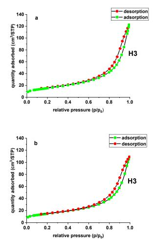
Figure 3. N<sub>2</sub> adsorption/desorption isotherms of  $X^{np}$  (a) and  $X^{np}$ -La(III) (b).
