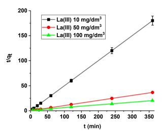
**Figure 8.** PSO plots of lanthanum(III) adsorption on  $X^{np}$  ( $c_0 = 10, 50, 100 \text{ mg/dm}^3$ , pH = 4, shaking speed 180 rpm, temperature 295 K).
