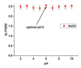
**Figure 10.** Effect of pH on adsorption of arsenic(V) on  $X^{np}$ -La(III) ( $c_0 = 10 \text{ mg/L}$ ; m = 0.1 g; t = 24 h, T = 295 K, shaking speed 180 rpm).
