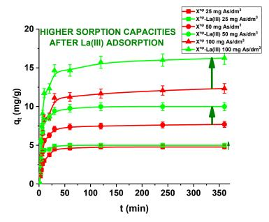
**Figure 11.** Sorption of arsenic(V) on  $X^{np}$  and  $X^{np}$ -La(III) as a function of time ( $c_0 = 25$ , 50 and 100 mg/dm<sup>3</sup>, pH = 6, shaking speed 180 rpm, temperature 295 K).
