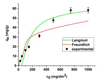
**Figure 15.** The Langmuir and Freundlich sorption isotherms of As(V) on X<sup>np</sup>-La(III) (pH 6, shaking speed 180 rpm, temperature 295 K).
