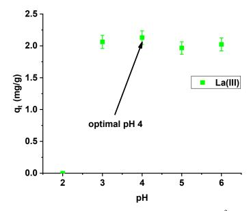
**Figure 6.** Effect of pH on lanthanum(III) adsorption on  $X^{np}$  ( $c_0 = 10 \text{ mg/dm}^3$ ; m = 0.1 g; t = 24 h).
