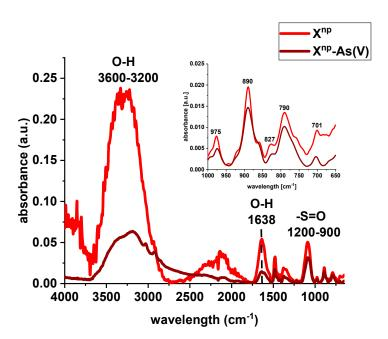
Figure 4. FTIR spectra of X<sup>np</sup> before and after sorption of As(V) ions.
