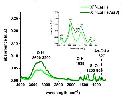
Figure 5. FTIR spectra of X<sup>np</sup>-La(III) before and after sorption of As(V) ions.
