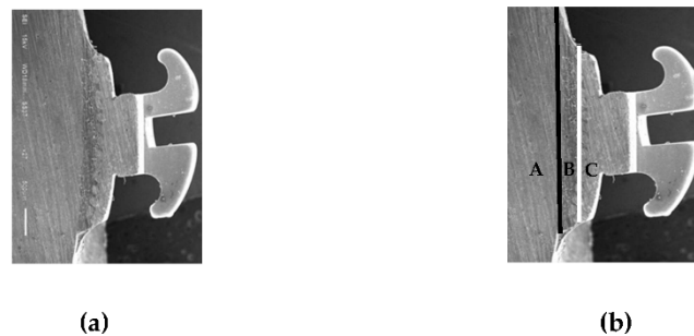
Figure 2. (a) Cross-sectional SEM image of the teeth with metallic bracket (original magnification \times 27 , bar represents 500 \mu\text{m} ); (b) A, enamel layer; B, adhesive layer; C, bracket base layer; black line, enamel–adhesive interface; white line, bracket base–adhesive interface.
