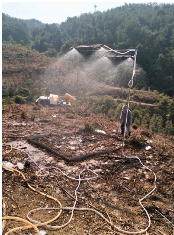
Fig. 3. The self-made device for the field-simulated experiment of rainfall.
