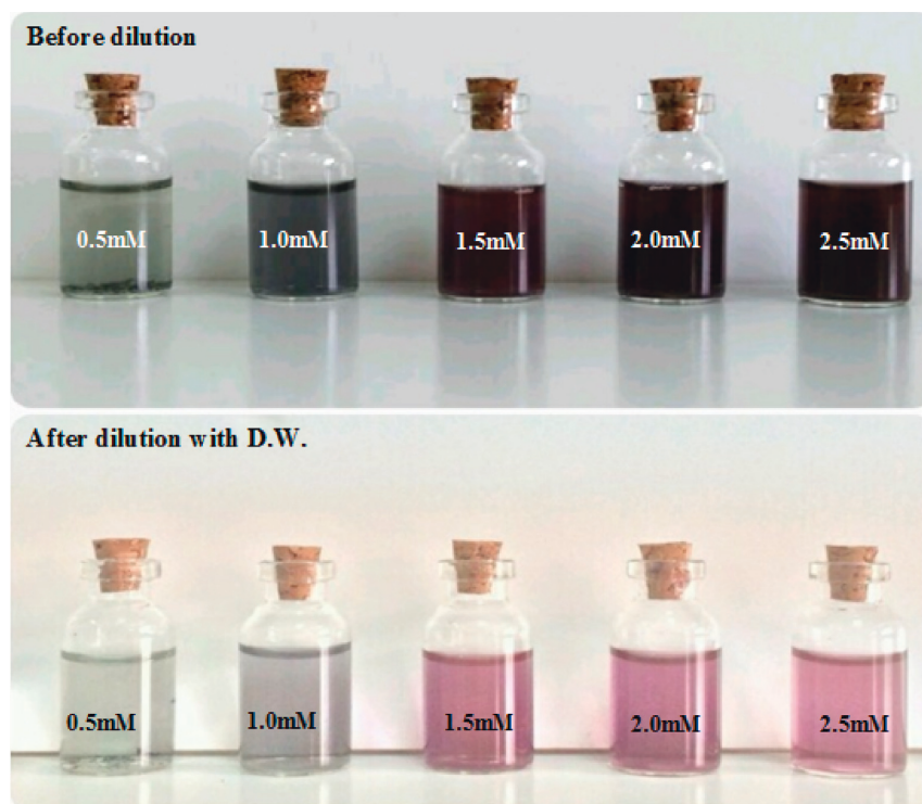
FIGURE 4: The pictures show the color changes after the process of reduction of \text{HAuCl}_4 solution to GNPs using different concentrations of \text{HAuCl}_4 solution (0.5, 1.0, 1.5, 2.0, and 2.5 mM) before and after dilution with distilled water.
