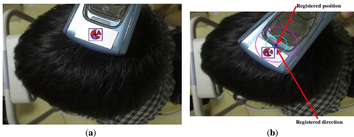
Figure 10. Detected center and direction of color marker and facial feature positions. (a) Detected center and direction of marker (registration mode in Figure 3); (b) Moving the diagnostic device to the registered position and in the direction of the marker (treatment mode in Figure 3); (c) Manually detected facial feature points.
