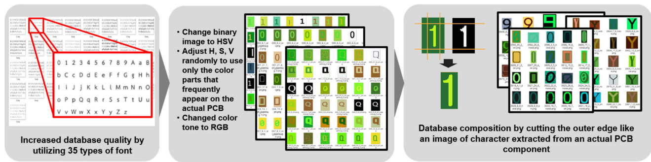
Figure 10. Creation of font data for colors appearing on PCB components in the real world.
